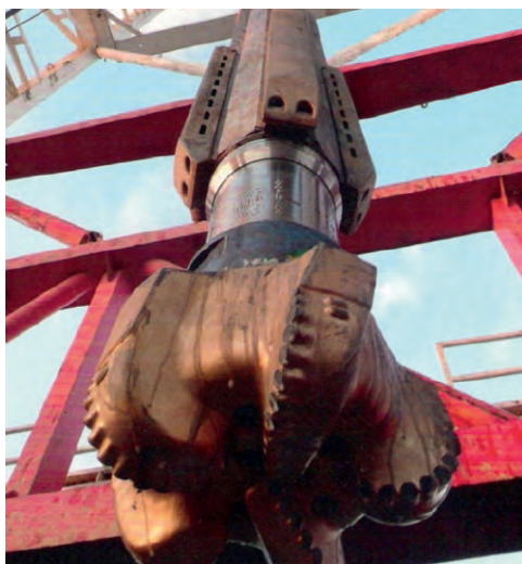
Figure 2 / Vertical boring with a rotary drilling tool.
