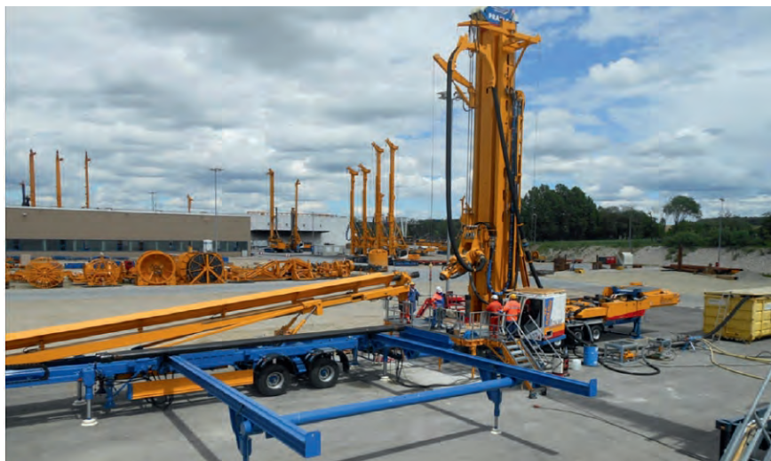
Figure 1 / Prakla-designed drilling rig with pipe handler for sinking rescue boreholes.
